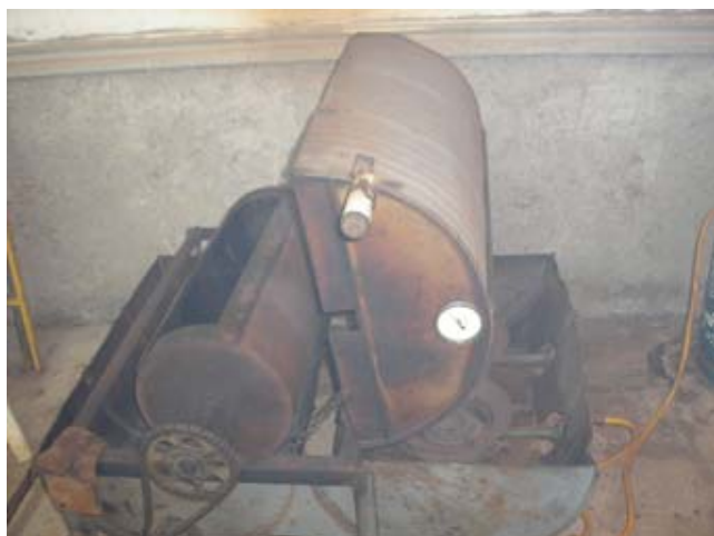
Picture 19: Improved hand-made roaster using gas
