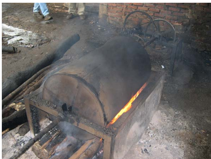
Picture 17: Hand-made roaster using wood
