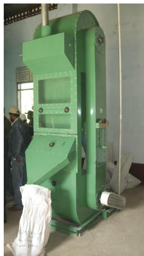
Figure 37. Catador used to clean coffee beans after hulling
